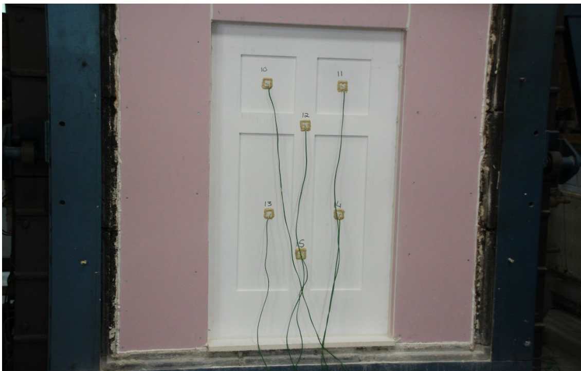
Image 2 – Before test, outside furnace
