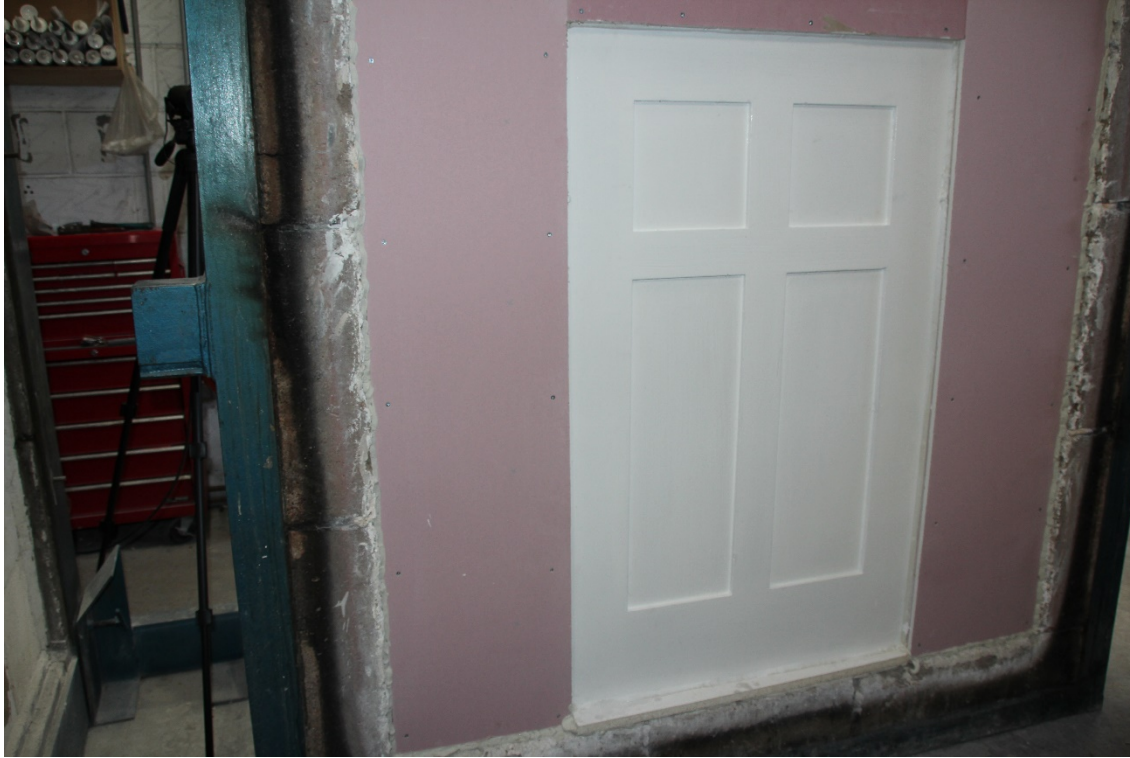
Image 1 – Before test, inside furnace
